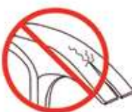
Crack in claw section
