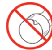
Chips or dents on face
