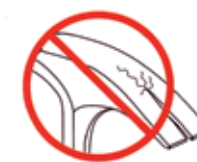
Crack in claw section
